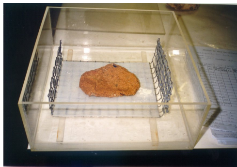
Figure 5 – Placement in a recipient with water
