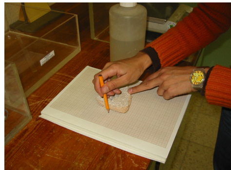
Figure 6 – Measurement of the absorption area
