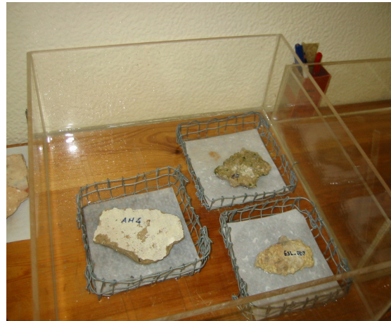
Figure 2 – Capillarity test for old mortars
