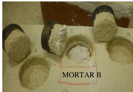
Fig.5 Specimens after pull-off test – mortars B.
