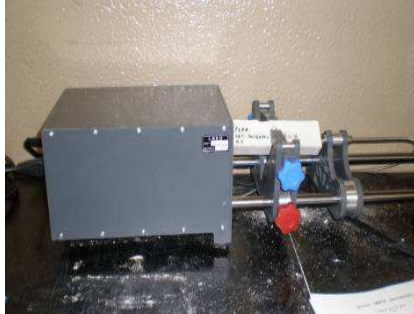
Fig. 3 Determination of dynamic modulus of elasticity.
