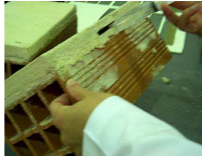
Fig.2 Specimens simulating the “detachment” between layers
