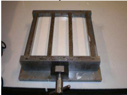
Fig.1 Preparation of prismatic specimens of grout mortars.
