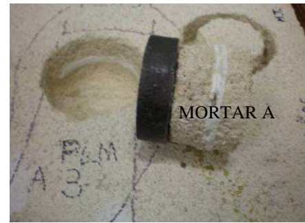
Fig.6 Specimens after pull-off test – mortars A.
