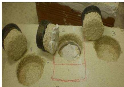
Fig. 4 – Pull-off test in laboratory
