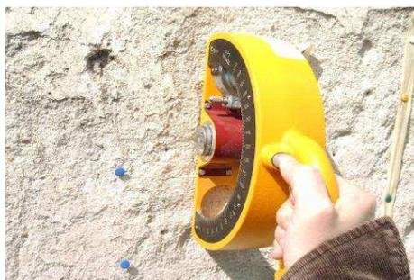
Fig. 3 – Test with Shmidt impact hammer on ancient lime mortar
