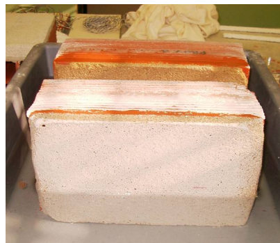
Figure 6 Degradation pattern of specimens after first cycle
