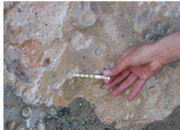
Fig. 3 In situ test for salt identification
