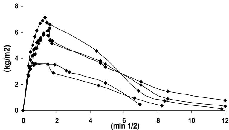
Figure 1: Absorption and drying curves on ancient rendering mortars.
