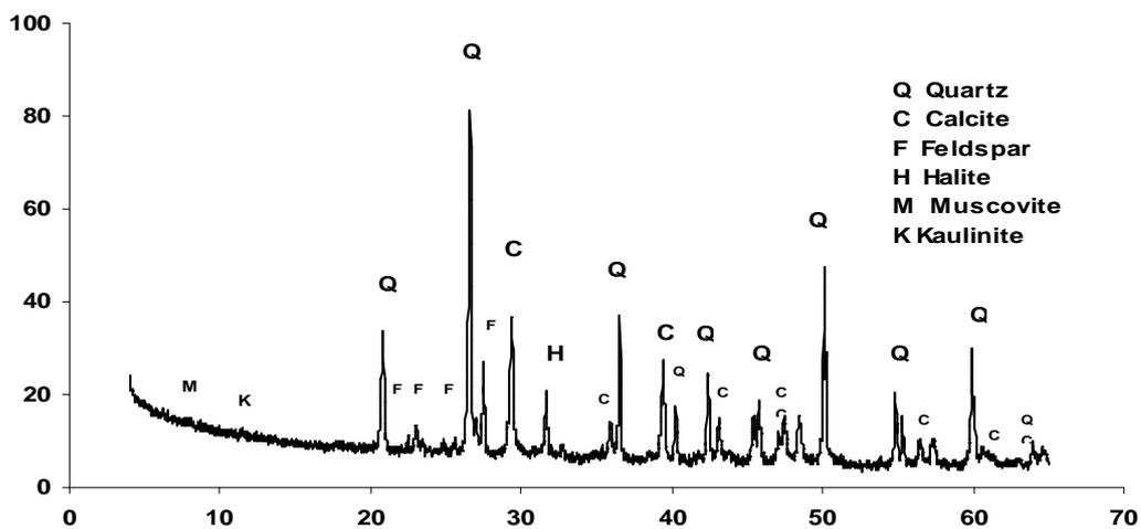
Figure 3: Typical XRD pattern from an old rendering mortar (MP5).
