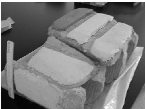
Figure 5. Mortars applied on adobe bricks.
