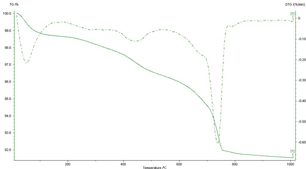
Figure 4: Typical DTA/TG analysis on an old rendering mortar (MP5).
