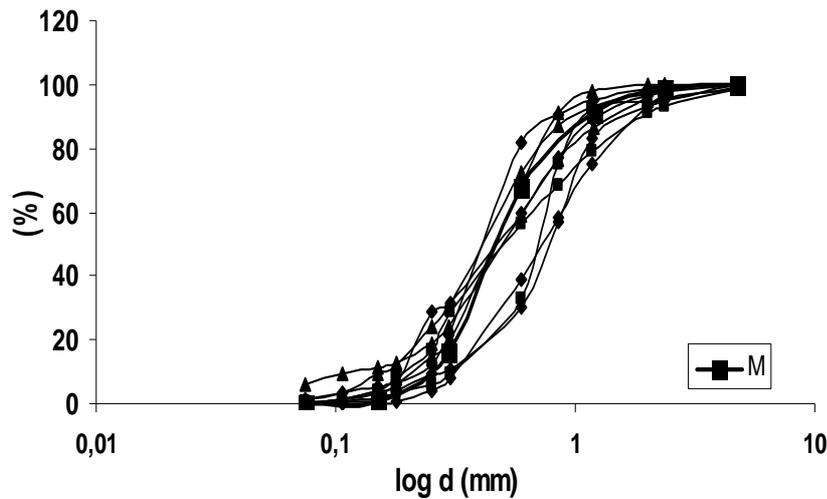
Figure 2. Particle size distribution of old (thin line) and adjusted aggregate for new mortars (thick line).
