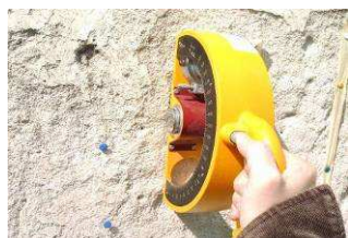
Fig. 3 – Test with Schmidt impact hammer on ancient lime mortar
