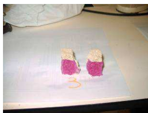
Fig. 4 – Test for evaluation of consolidation deepness with phenolphthalein agent
