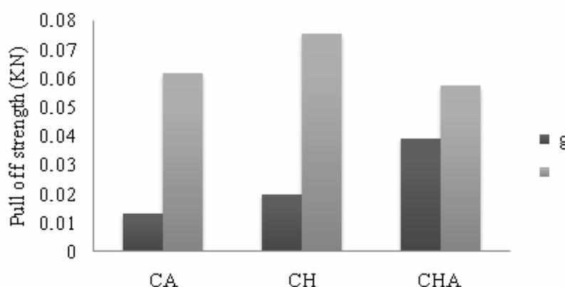
Figure 9: Results from pull off strength tests on brick samples (Darker bars represent values from areas with grout (g) and brighter grey bars represent areas without the grout).
