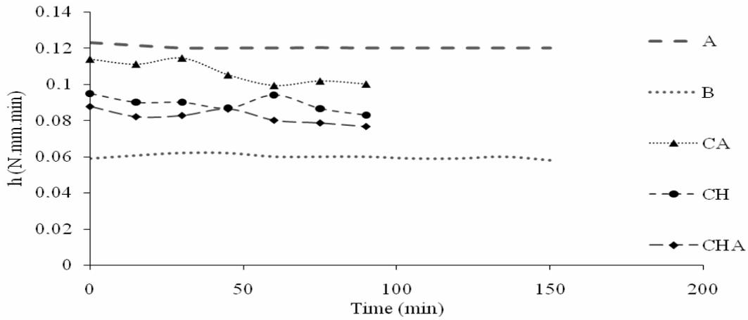
Figure 3: Variation of h parameter as a function of testing time for the different grout composition.
