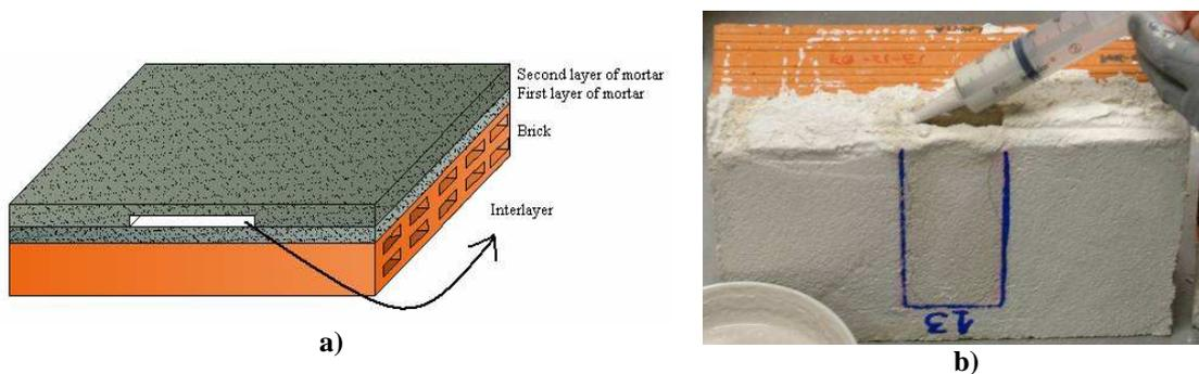
Figure 2: a) Brick samples scheme; b) Grout application on a brick sample
