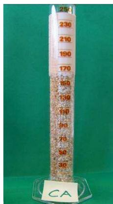
Figure 5: Injectability test made on the CA formulation.
