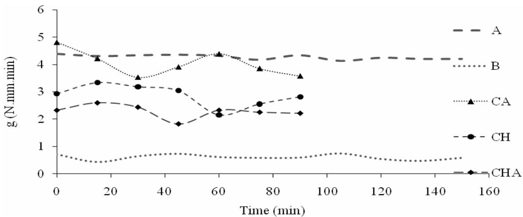
Figure 4: Variation of g parameter as a function of testing time for the different grout composition.
